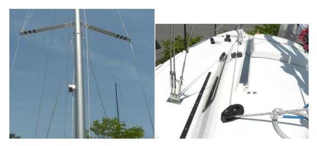
Figure 1. Left photo shows the illegal after-market reverse cam cleat mounted on the mast. Right photo shows the allowed configuration with a single 150 cam-cleat mounted on the cabin top. The three shroud turnbuckles shown in the photo are the ones installed at the factory any deviation from this configuration is illegal.
