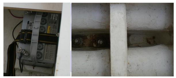
Figure 4. The picture on the left shows the battery and the picture on the right shows the bilge that is dry. We will inspect the known areas where water collects.
