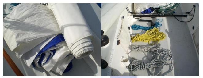
Figure 3. The picture on the left show the main and spinnaker without storage bags in the cockpit of the boat being weighed. The picture on the right shows the jib sheets, tack line, spin sheets, backstay line and winch handle. The mainsheet is attached to the boom and the traveler control line is rigged. All other control lines can be in their functional position such as the halyards.
