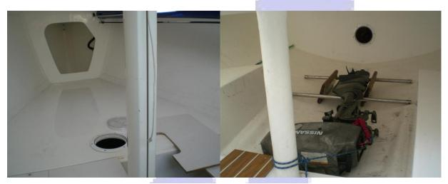
Figure 2. The two pictures above show the interior of a J80 ready to be weighed. The airtight covers are open and the cover to the battery box is open. The stairs do not have to be attached in their normal location but on board. Water tends to collect in the small forward compartment in the left photo and in the airtight compartments.
